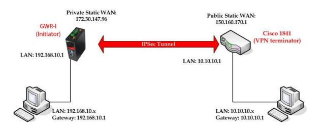
Figure 84 - IPSec tunnel between GWR-I Router and Cisco Router
