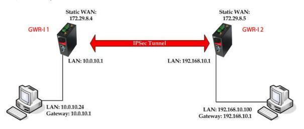
Figure 63 - IPSec tunnel between two GWR-I Routers
