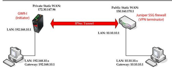
Figure 90 - IPSec tunnel between GWR-I Router and Cisco Router
