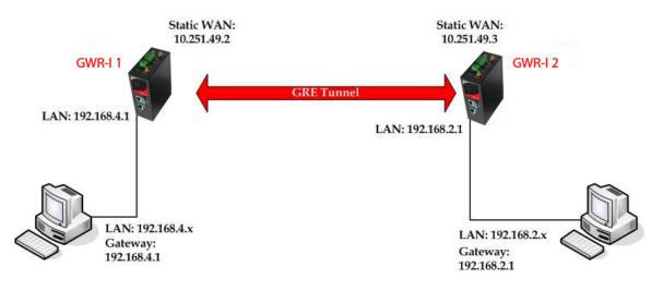
Figure 52 - GRE tunnel between two GWR-I Routers
