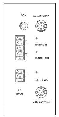
Figure 3 – GWR-I Router top panel side
