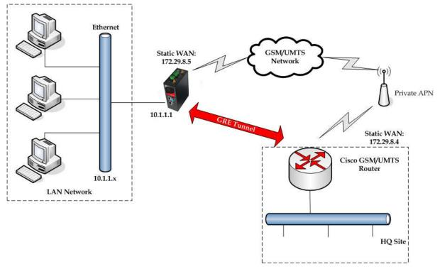
Figure 59 - GRE tunnel between Cisco router and GWR-I Router
