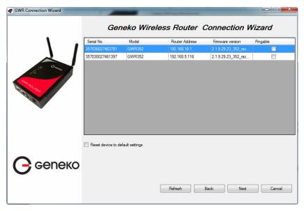
Figure 46 - Connection Wizard - Router Detection
