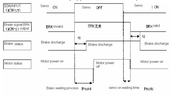
t1, t2: determined by external relay and brake loop move time
