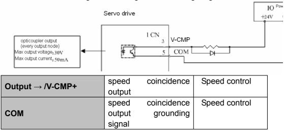
It refers to output signal of input speed reference and speed coincidence of actual motor rotation. When output status at low is active:
