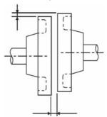
Measure this at four quartering positions of a cycle. The difference between the maximum and minimum measured value must be less than 0.03mm. (Rotate together with shaft connectors)
