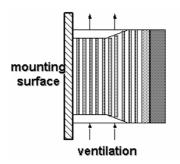
A cooling fan can be mounted for forced-air cooling of the servo drive at request.
