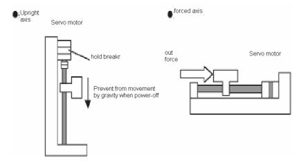
Make sure servomotor is mechanically separated before confirming action of servomotor and brake sticking(holding brake) . If all the parts are moving well, connect servo motor to the machine.
