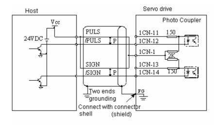
Example 3 (When host device is open collector output subject to 12VDC or 5VDC signal power)
