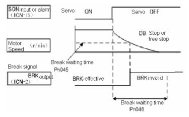
For a running brake sticking motor, if S-OFF is caused by variation of /S-ON or alarm occurrence, it's required to set brake waiting speed of servomotor or brake waiting time.
