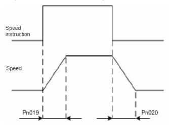
Pn019 and Pn020 are linear acceleration/deceleration time. In the event of rather large impact which may occur because linear acceleration/deceleration time are applied, Pn021 can be selected and set to get a smooth running.
