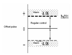
When Pn047 is set to 1, if the range of error counter overflow(Pn031) is set too small, alarm A.06 may occur when running at high speed.
