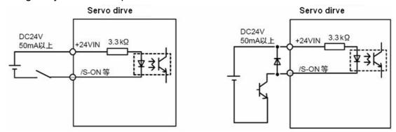
If the relay contact input is used, the relay must be suitable for tiny electric current, otherwise it causes signal receiving faults easily.
