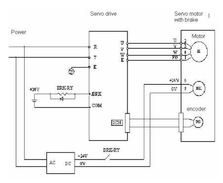
BRK-RY: brake sticking control relay
