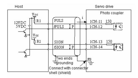
The right current limiting resistor R1 should be used according to current requirements (i  $=10\sim15\text{mA}$ ):
