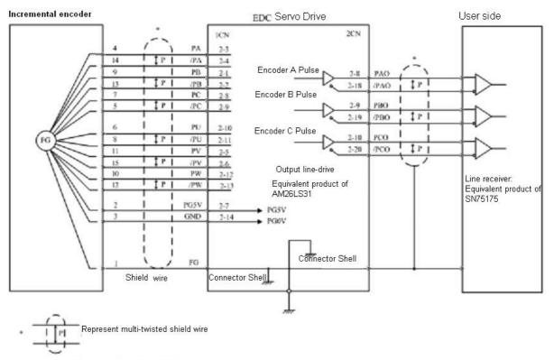
Ps: 1 The sequence No. of encoder pin's corresponding relation with signal will change because of different types of motors.
