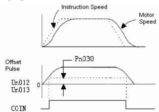
Un012: error pulse counter low position monitoring Un013: error pulse counter high position monitoring When output is active at low level:
