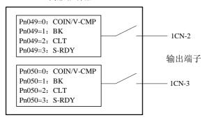
Following table shows the pin number definition for Pn049 (correspond to pin 1CN-2 output), Pn050 (correspond to pin 1CN-3output).
