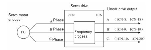
Divide pulse frequency of servomotor encoder(PG) and output according to pulse number setting.
