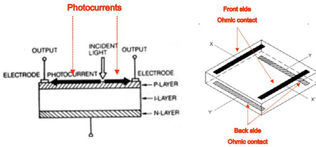
Fig. 8. The duolateral PSD sensor
