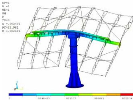
Fig. 5. Deformations of the PhoCUS structure
