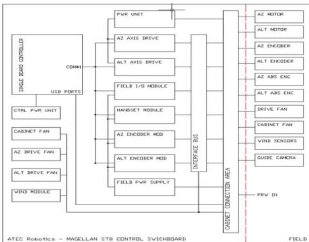
Fig. 3. The control system block scheme
