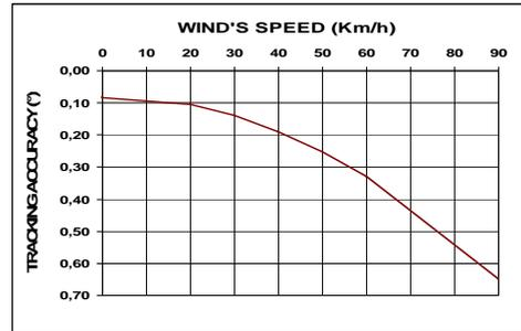
Fig. 6. Module misalignments vs. wind velocity
